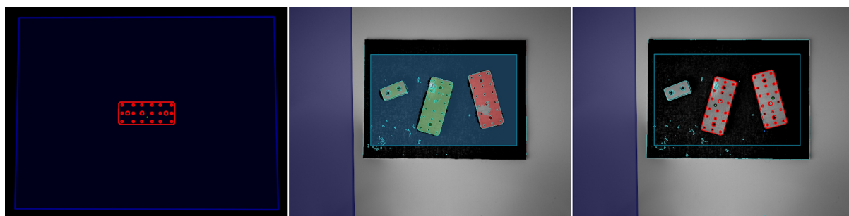
Fig. 6.19: “Template”, “Intermediate Result” and “Result” image streams of the SilhouetteMatch module as shown in the Web GUI for a detection with object_plane_detection set to true
