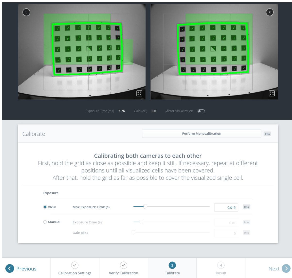
Fig. 6.33: Stereo calibration: Hold the grid as close as possible to fill all visualized cells
