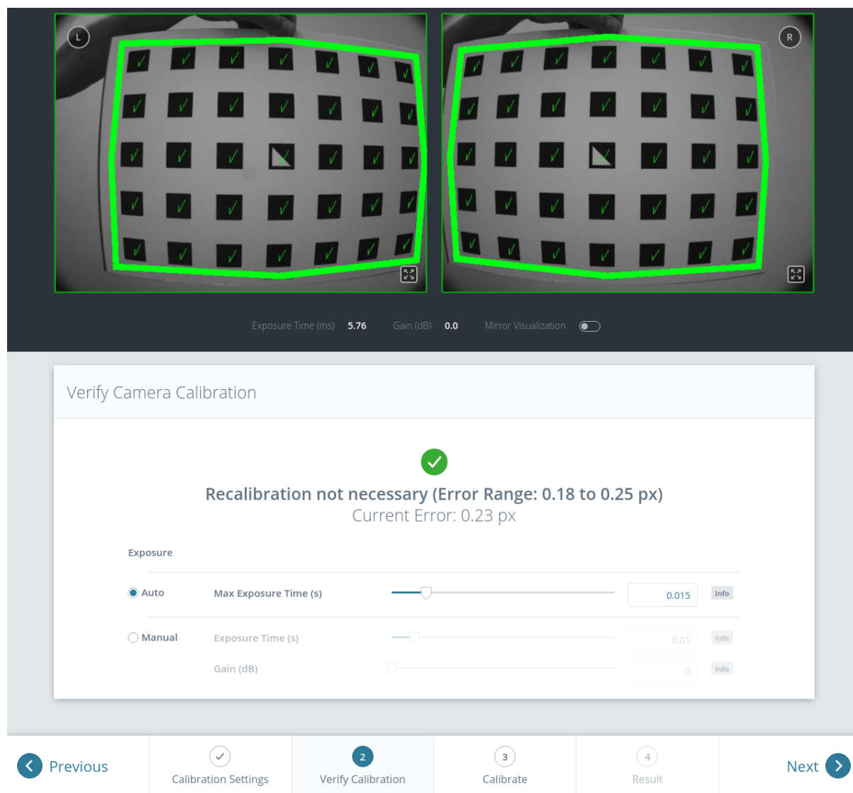
Fig. 6.31: Verification of calibration
