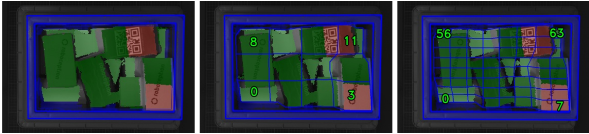
Fig. 6.9: Visualizations of the load carrier filling level: overall filling level without grid (left), 4x3 grid (center), 8x8 grid (right). The load carrier content is shown in a green gradient from white (on the load carrier floor) to dark green. The overfilled regions are visualized in red. Numbers indicate cell IDs.
