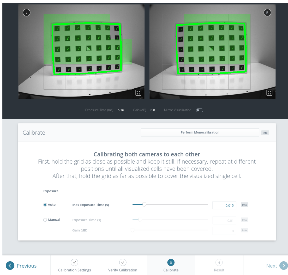
Fig. 6.34: Stereo calibration: Hold the grid as close as possible to fill all visualized cells
