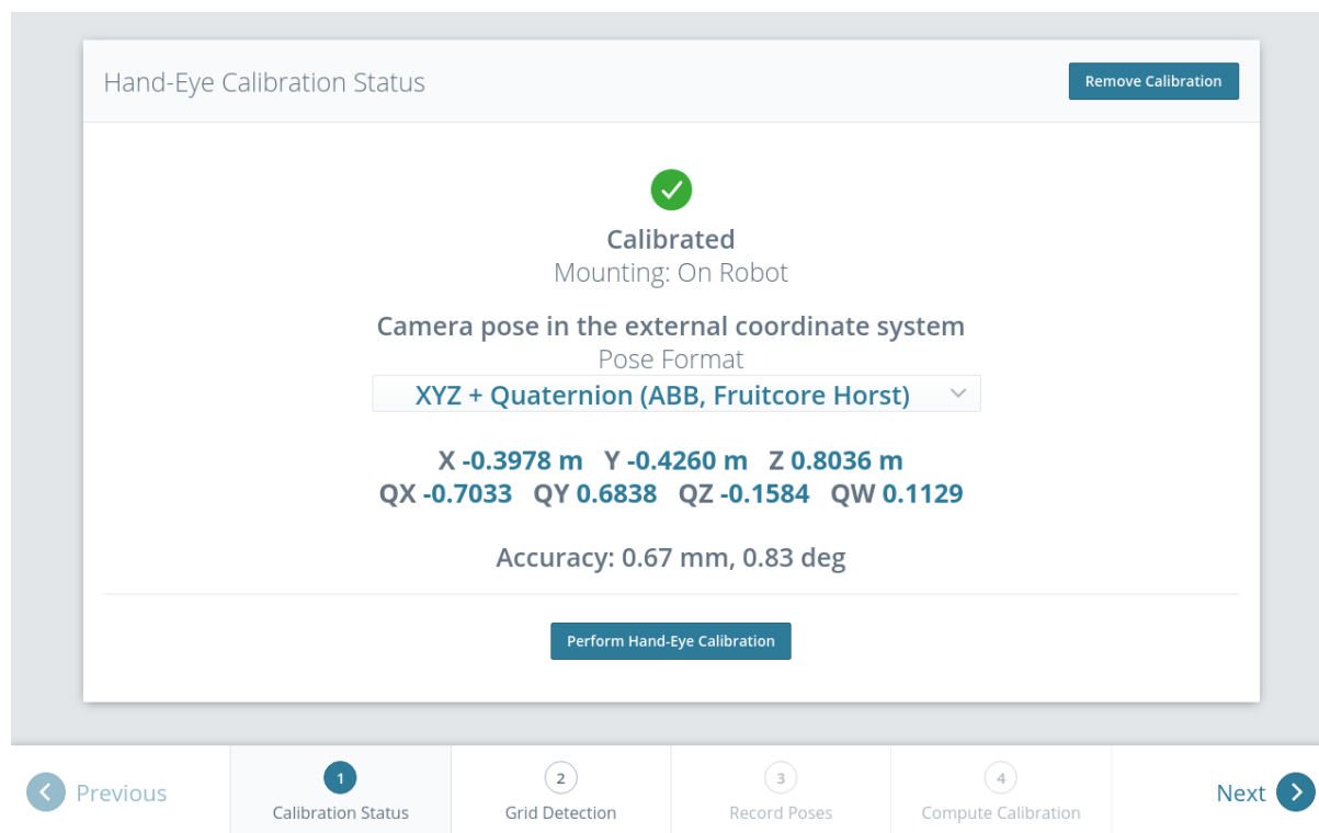
Fig. 6.25: Current status of the hand-eye calibration in case a hand-eye calibration is saved
