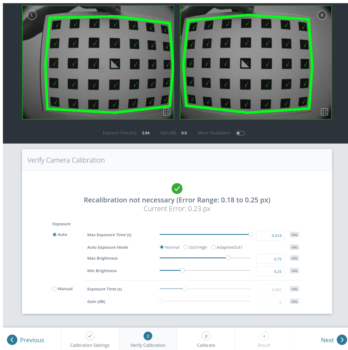
Fig. 6.33: Verification of calibration
