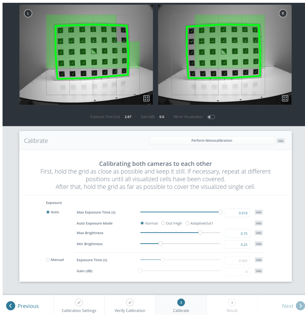
Fig. 6.35: Stereo calibration: Hold the grid as close as possible to fill all visualized cells
