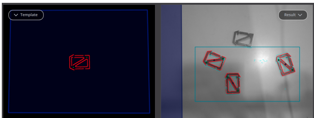
Fig. 6.22: Result image of the SilhouetteMatch module as shown in the Web GUI
