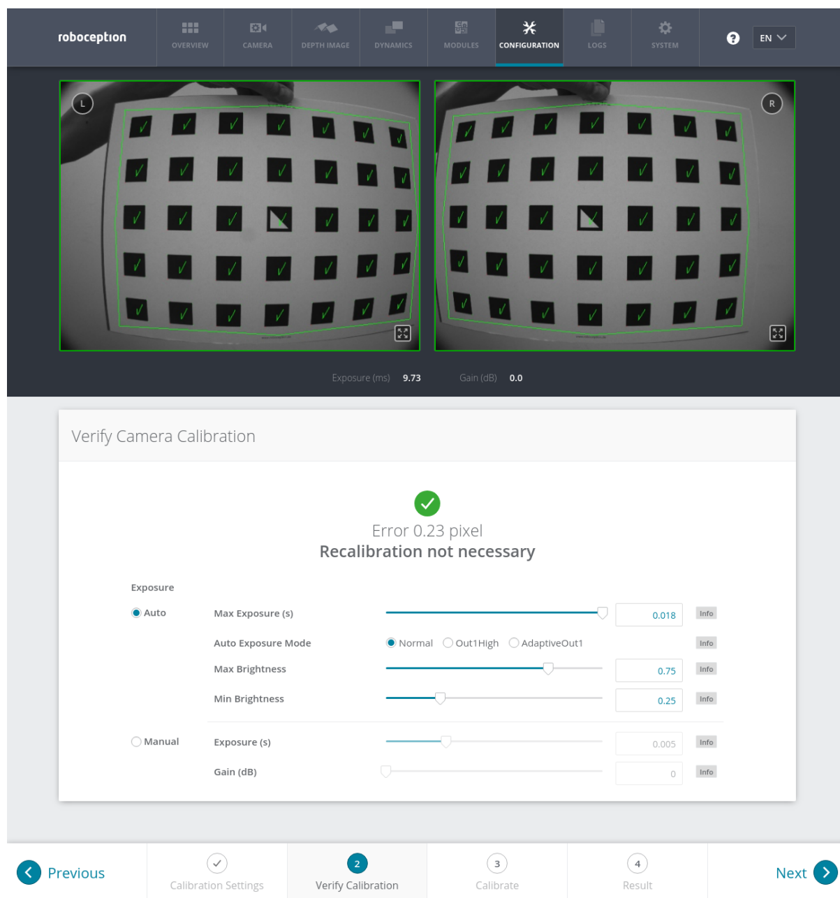
Fig. 6.38: Verification of calibration
