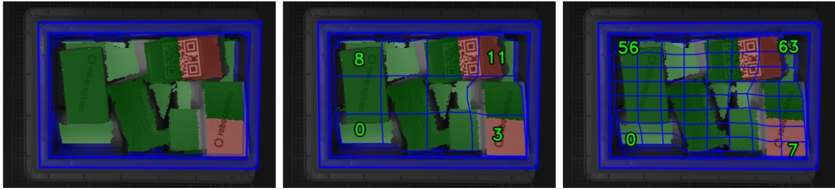
Fig. 7.10: Visualizations of the load carrier filling level: overall filling level without grid (left), 4x3 grid (center), 8x8 grid (right). The load carrier content is shown in a green gradient from white (on the load carrier floor) to dark green. The overfilled regions are visualized in red. Numbers indicate cell IDs.
